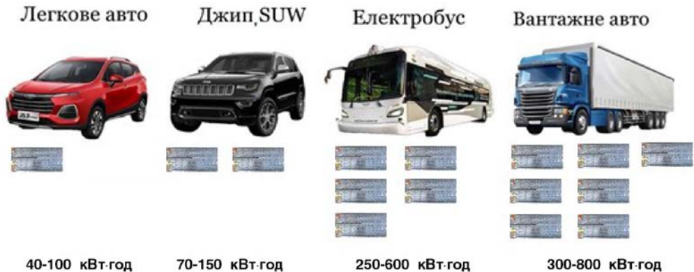
Figure 2. The number of lithium-ion modular sectional batteries in different types of cars
