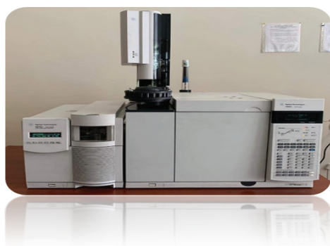
Agilent «GC-7890A» 7890A Gas Chromatograph combined with «MSD-5975C» Gas Chromatograph/Mass Selective Detector (GC/MSD) system
