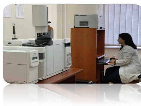
Agilent «GC-7890A» 7890A Gas Chromatograph combined with «MSD-5975C» Gas Chromatograph/Mass Selective Detector (GC/MSD) system
